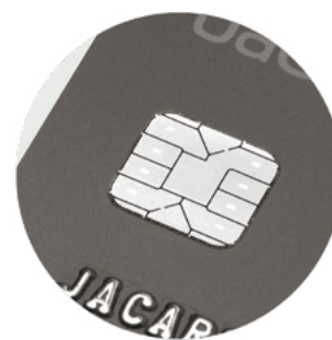
After 10,000 insertion cycles (JCR-721 reader with Landing contact group and Microlift™)
