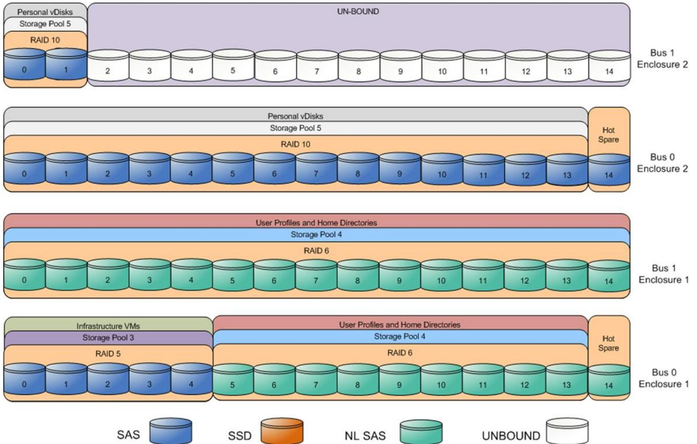
**Figure 4. VNX5300 – optional reference architecture physical storage layout**
