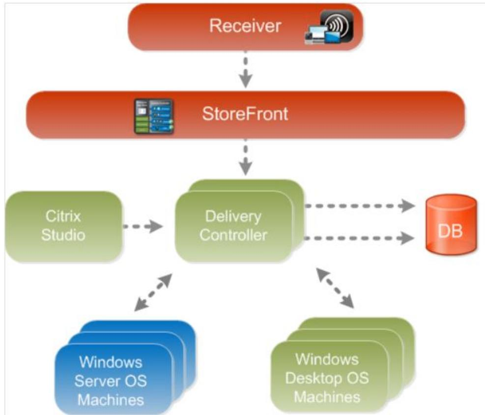
Figure 9. Citrix XenDesktop 7 architecture components
