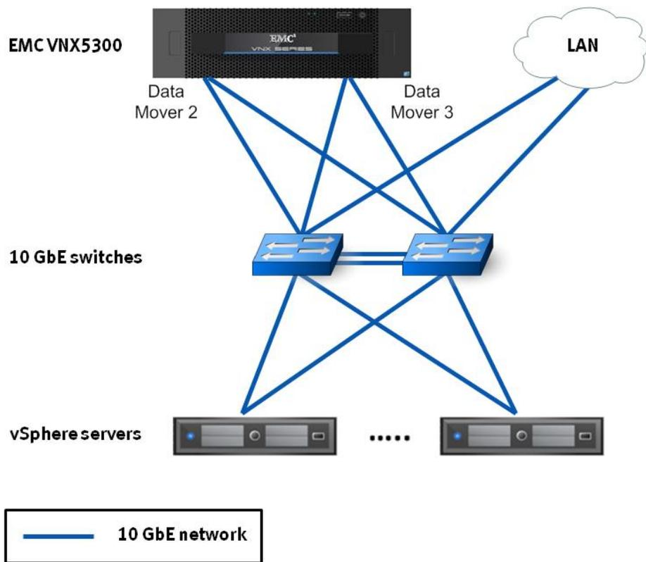
Figure 5. Network layout diagram for NFS variant
