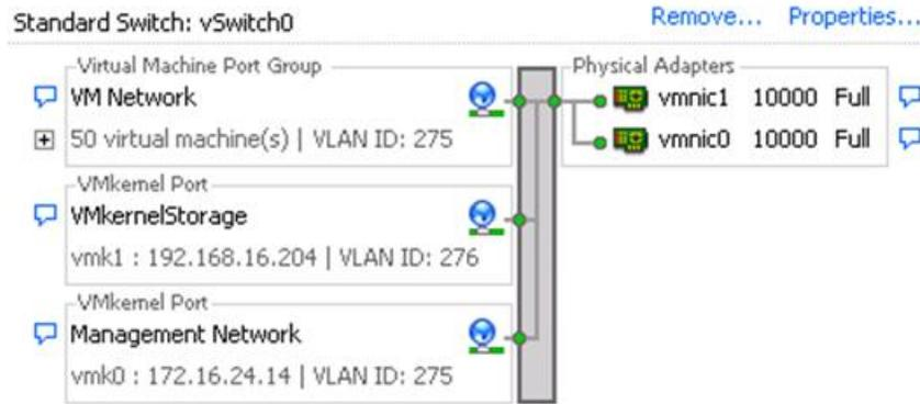
**Figure 7. vSwitch configuration in vCenter Server**
