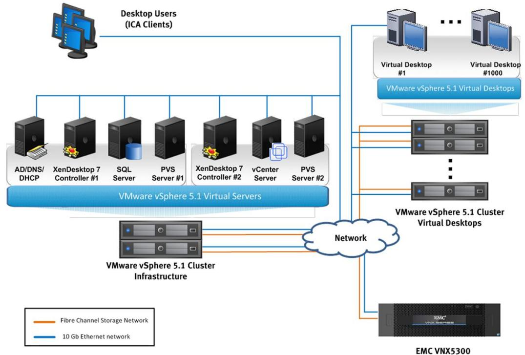
**Figure 2. Logical architecture for 1,000 virtual desktops – FC variant**
