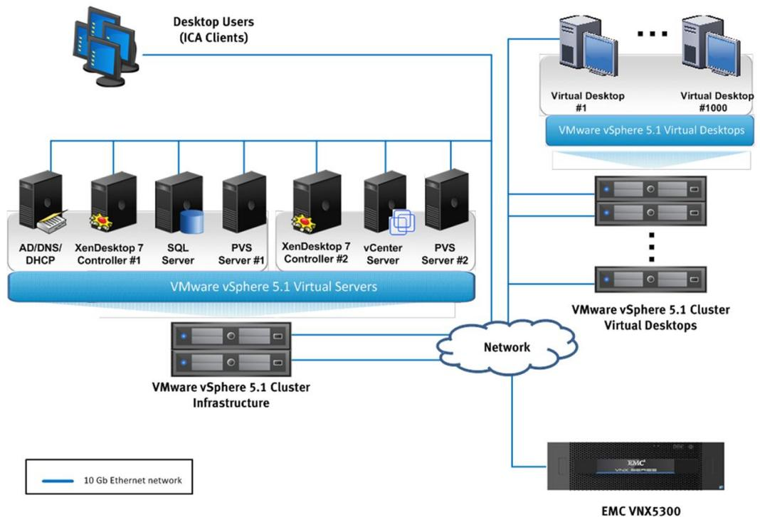
Figure 1. Logical architecture for 1,000 virtual desktops – NFS variant
