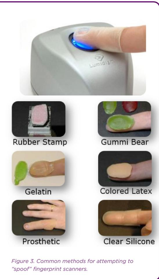
Figure 3. Common methods for attempting to “spooF” fingerprint scanners.
