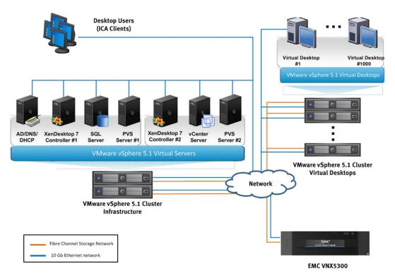
Figure 2. Logical architecture for 1,000 virtual desktops – FC variant
