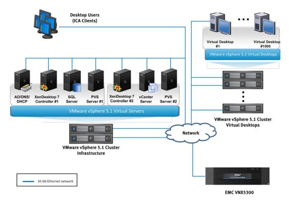
Figure 1. Logical architecture for 1,000 virtual desktops – NFS variant
