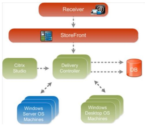
Figure 9. Citrix XenDesktop 7 architecture components
