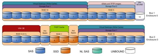
Figure 3. VNX5300 – core reference architecture physical storage layout
