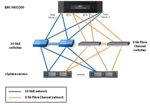
Figure 6. Network layout diagram for FC variant
